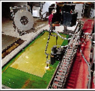
Cutting/Burning Table Greenheck's DNC plasma cutter ensures cutting accuracy.
