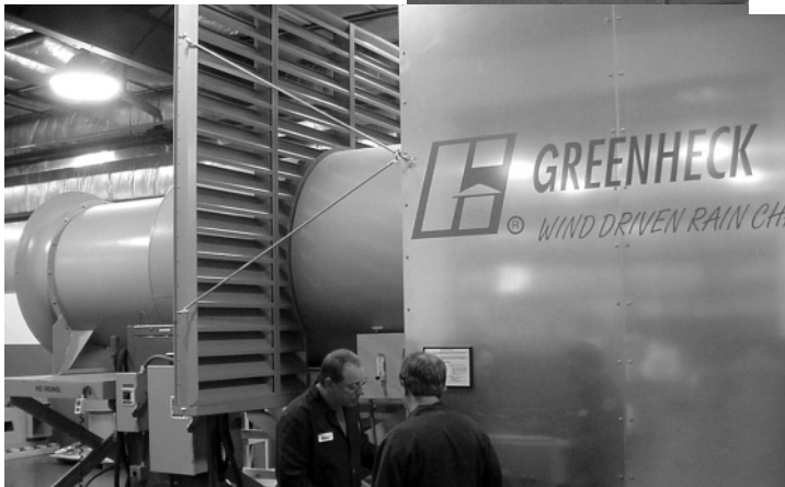
Damper being put through the test cycle on the wind drive rain tunnel
