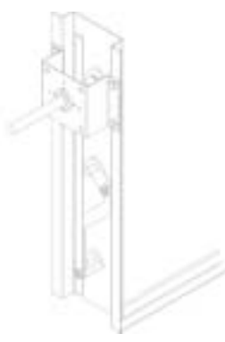
Extended Operating Shaft
